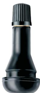
**VÁLVULA PARA PNEUS SEM CÂMARA**
